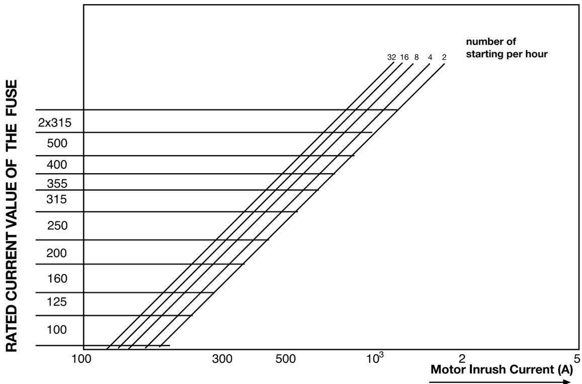
**MV FUSE PROTECTION FOR MOTORS WITH INRUSH PERIOD NOT EXCEEDING 30 SECONDS**
