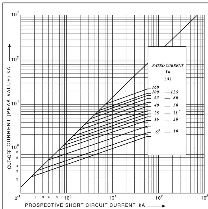
The cut-off current of our h.v. h.b.c. fuse links, which can be taken from the diagram, are a function of the prospective short-circuit current (r.m.s. value of the symmetrical component) and of the rated current.
